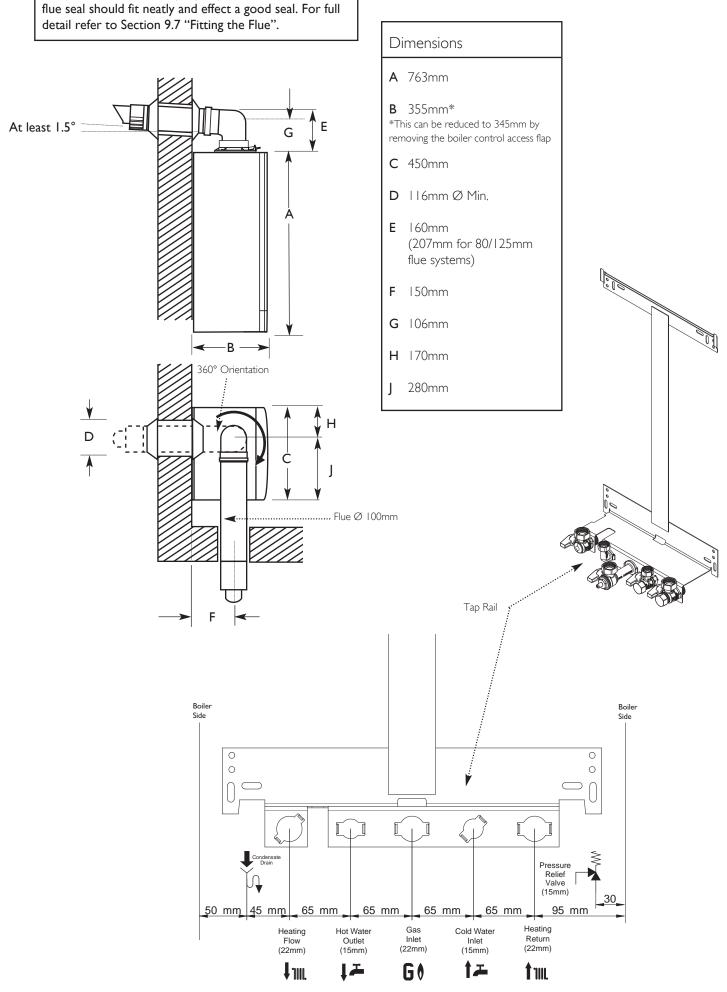
Note: There must be no part of the air duct (white tube) visible outside the property after installation. The
