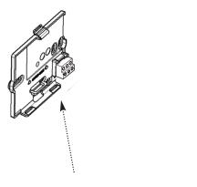
Boiler Wiring Terminal M2 Low Voltage Terminal Block
