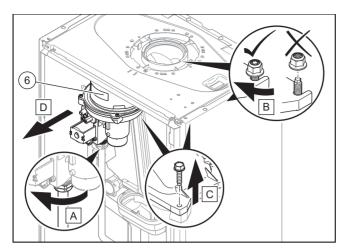
9. Remove the gas-air mixture unit (6).
