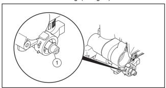
Regulate the pressure using the adjusting screw (1).
